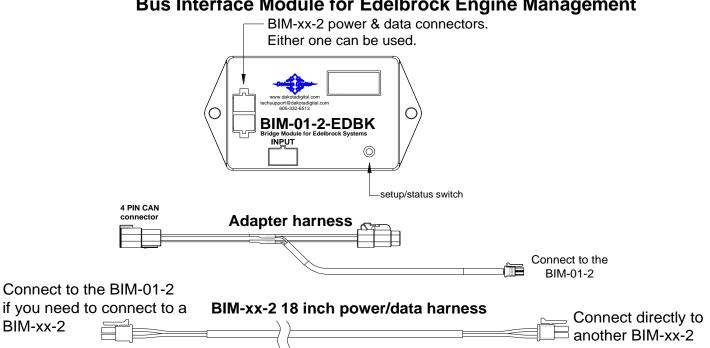
This Bus Interface Module is designed to read engine information from specific Edelbrock CAN bus enabled EFI units which currently includes: Pro-Flo 4 EFI system with v53 or later. The module is connected to the Edelbrock device main harness through one of the adapter harnesses that are included within this kit.
