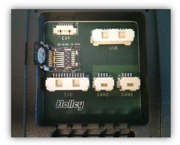
Figure 3. Insert micro-SD card
