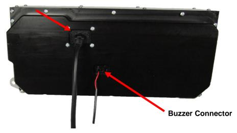
2. Mount the RTX system to the dash using the stock screws. Make sure to partially thread all screws before final torqueing to ensure proper alignment for all mounting points.
