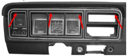
1b. Finally, remove the four (4) mounting screws holding the cluster to the dash. Retain these screws for reassembly.
