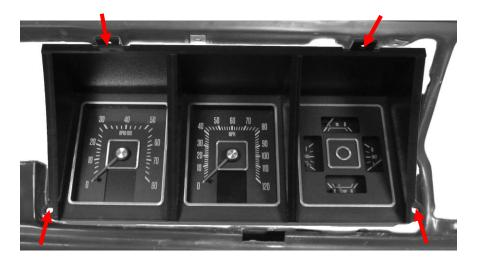
4. Refer to the main manual for wiring instructions and re-install the stock bezel in reverse order using all stock hardware to complete the RTX installation.
