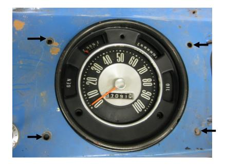
2. Remove these four screws to separate the bezel from the gauges and set aside for reassembly.
