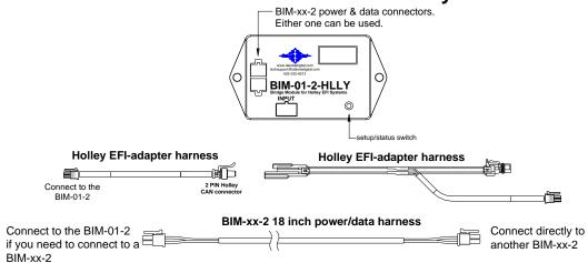
This Bus Interface Module is designed to read engine information from specific Holley EFI kits. These kits include Holley Terminator, HP, Sniper, Dominator and Terminator X. The module is connected to the Holley EFI through the CAN-bus plug on the EFI harness. Depending on your EFI module you may have a 2-pin or 4-pin CAN connector. We supply EFI adapter harnesses that will allow you to connect with your particular kit.
