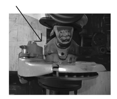
Caliper mounting should be at the 9 o' clock position on the passenger side and the 3 o' clock position on the driver side.
