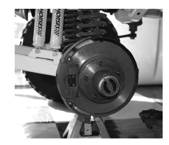
Be sure to mount calipers with the bleed screws up. The brake hoses should be mounted up and then into the bracket on the front end. DO NOT mount the hose back and into the bracket because it could rub on the tire or wheel. Double check hose install by turning wheels full right and full left while watching the hose. Make sure there is no interfearance anywhere.
