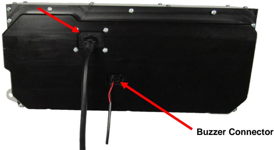
2. Mount the RTX system to the dash using the stock screws. Make sure to partially thread all screws before final torquing to ensure proper alignment for all mounting points.
