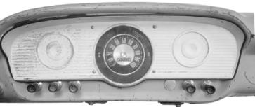
2. Remove these four screws to separate the bezel from the gauges.
