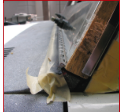
9. As you fold the windshield up for the first time, you need to make a final left-right alignment (where the finger is pointing) so the lip of the cowl will clear the frame. This is difficult to explain but easy to see in practice. Our fit was exactly perfect, but you can bend the sheet metal in or out if you need 1/16" or so more room. The hinge should be positioned so it sticks out a little. The directions are clear about this.
