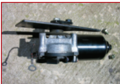
6. Now we begin with the new installation. We put all the linkage and wiper motor in place and positioned the entire windshield assembly on the Bronco so we could see exactly where the defroster metalwork needs to be cut to clear the motor.
