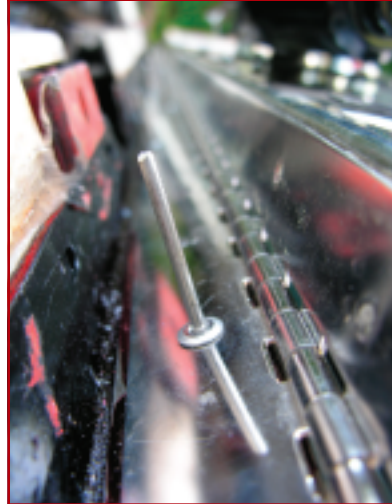
12. When you have everything exactly in place, it is time to use the provided stainless steel rivets to attach the lower hinge to the body. This was probably the second hardest part of the job for me. I only had a cheap rivet gun for aluminum rivets, so I went out and bought a beefy unit for stainless steel. It worked fine, but you have to WORK to get that rivet to finally pop off. Getting those last rivets installed made me whimper. If you are not into weight lifting, you might want to borrow a power rivet gun for an hour.
