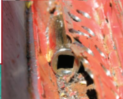
3. My windshield frame hadn't been lowered in some 20 years of off-road use and there was so much grime under the hinge that an hour or so was needed just to brush and wash the area clear in preparation to cut out the old hinge.
