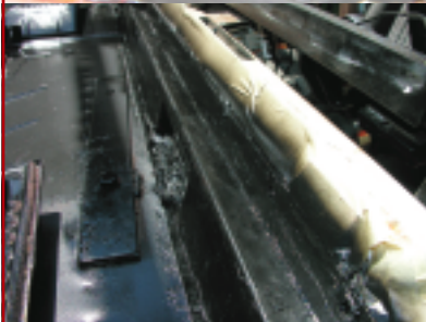
5. After all the cutting and drilling, we spent some extra time to clean, de-rust, fill in and seal the entire body area below the hinge. You won't be able to get back in here for a long time, so it's worth the extra preventative maintenance.
