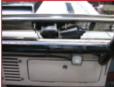
7. Gary has neatly packaged all the linkage recessed in the frame completely out of the way. The motor, however, needs to fit in an area just above the glove box. Dimensions come with the instructions, but we measured carefully so we would not cut out any more than needed. Once you have marked everything, the actual cutting was easy with a combination of a saber saw and a sawzall. As always, measure twice and cut once.
