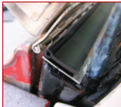
13. Now you are in the home stretch. Just do the obvious things like installing the hinge gasket and bolting anything you took off - like the hood - back in place.
