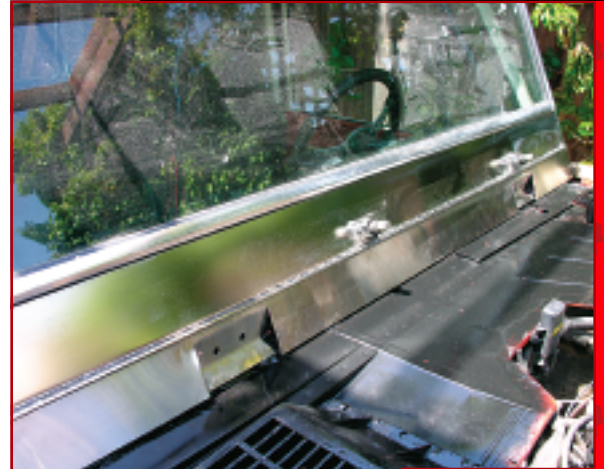
12. When you have everything exactly in place, it is time to use the provided stainless steel rivets to attach the lower hinge to the body. This was probably the second hardest part of the job for me. I only had a cheap rivet gun for aluminum rivets, so I went out and bought a beefy unit for stainless steel. It worked fine, but you have to WORK to get that rivet to finally pop off. Getting those last rivets installed made me whimper. If you are not into weight lifting, you might want to borrow a power rivet gun for an hour.
