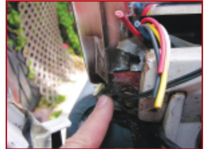
9. As you fold the windshield up for the first time, you need to make a final left-right alignment (where the finger is pointing) so the lip of the cowl will clear the frame. This is difficult to explain but easy to see in practice. Our fit was exactly perfect, but you can bend the sheet metal in or out if you need 1/16" or so more room. The hinge should be positioned so it sticks out a little. The directions are clear about this.
