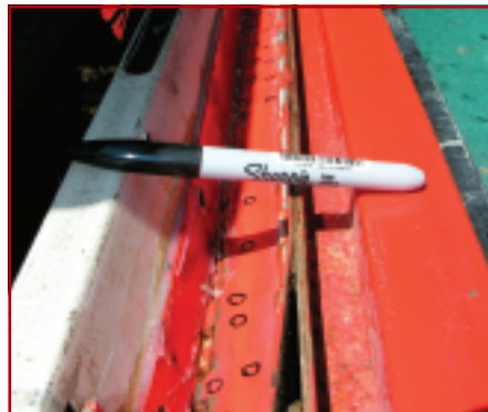
3. My windshield frame hadn't been lowered in some 20 years of off-road use and there was so much grime under the hinge that an hour or so was needed just to brush and wash the area clear in preparation to cut out the old hinge.
