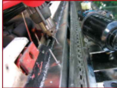
12. When you have everything exactly in place, it is time to use the provided stainless steel rivets to attach the lower hinge to the body. This was probably the second hardest part of the job for me. I only had a cheap rivet gun for aluminum rivets, so I went out and bought a beefy unit for stainless steel. It worked fine, but you have to WORK to get that rivet to finally pop off. Getting those last rivets installed made me whimper. If you are not into weight lifting, you might want to borrow a power rivet gun for an hour.
