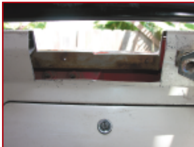
5. After all the cutting and drilling, we spent some extra time to clean, de-rust, fill in and seal the entire body area below the hinge. You won't be able to get back in here for a long time, so it's worth the extra preventative maintenance.
