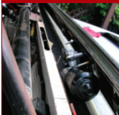
7. Gary has neatly packaged all the linkage recessed in the frame completely out of the way. The motor, however, needs to fit in an area just above the glove box. Dimensions come with the instructions, but we measured carefully so we would not cut out any more than needed. Once you have marked everything, the actual cutting was easy with a combination of a saber saw and a sawzall. As always, measure twice and cut once.
