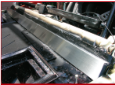
11. I added an extra piece of thin stainless steel from under the windshield hinge and down behind the hood hinge. This is NOT part of the kit, but I liked the idea of continuing the stainless steel look down behind the hood. I just went to a local Fab shop and had them cut and bend to the right size, then did a little custom trimming for the hood hinges. Did I mention to measure twice and cut once?
