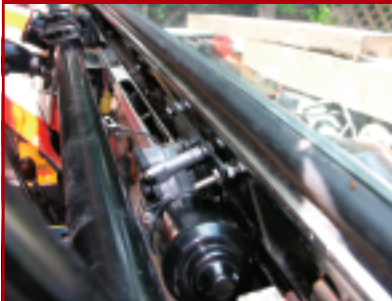
10. When you fold the frame up the first time you can see exactly where the motor bolts go. On this prototype I took a different path and cut a smaller opening and just drilled a hole for the one bolt closest to the driver. This approach as photographed is no longer required because in the production frames, the new wiper mount does not require the trimming of the heater duct unless you have a 66. The mount is shorter but it will still need clearance in the dash almost exactly as shown here.
