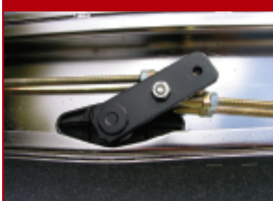
6. Now we begin with the new installation. We put all the linkage and wiper motor in place and positioned the entire windshield assembly on the Bronco so we could see exactly where the defroster metalwork needs to be cut to clear the motor.
