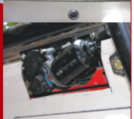
8. These photos show the cut away area from both sides, and where the motor fits. Note that I cut as little as possible into the plastic defroster vent contained inside the sheet metal. Only an inch or two was removed, and that left the air flow essentially unchanged from stock. While I'm happy with this approach, it isn't quite as the instructions describe the job and does require you do some different spacing of the motor on its bracket to sandwich everything in. I've discussed this with Gary and he will decide in production how best to recommend you do your installation. Note also that if you have a dash pad, it isn't hard to hollow it out on the back side so it fits over the motor and nearly hides it. All in all, the new motor actually tucks in and is less intrusive than Ford's designers cooked up back in the 1960.
