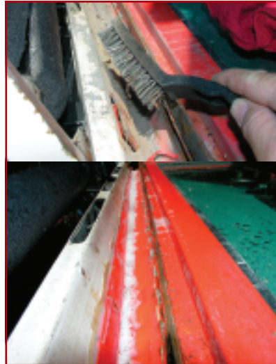
3. My windshield frame hadn't been lowered in some 20 years of off-road use and there was so much grime under the hinge that an hour or so was needed just to brush and wash the area clear in preparation to cut out the old hinge.
