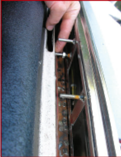
10. When you fold the frame up the first time you can see exactly where the motor bolts go. On this prototype I took a different path and cut a smaller opening and just drilled a hole for the one bolt closest to the driver. This approach as photographed is no longer required because in the production frames, the new wiper mount does not require the trimming of the heater duct unless you have a 66. The mount is shorter but it will still need clearance in the dash almost exactly as shown here.
