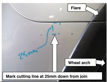
2. Using a non permanent marker, measure and mark a point 25mm (1") down from the bumper and fender join both sides of vehicle
