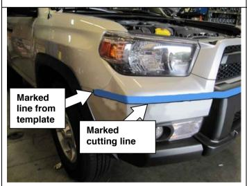
9. Apply 50mm masking tape along the top side of the cutting line right across the bumper as shown.
