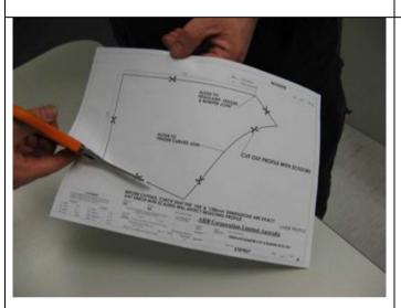
5. Using scissors accurately cut out the bumper cutting template along designated bumper cutting line as shown.
