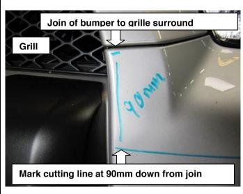
Mark a position for the cutting line at 90mm (3 ½") down from bumper to grille surround join inboard of headlamp as shown, repeat on other side of vehicle
