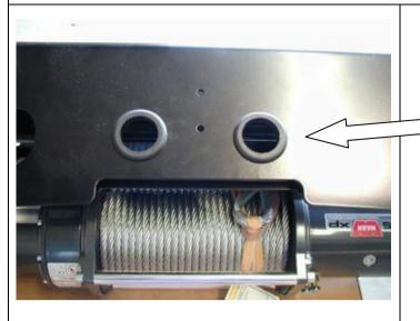
62. Insert the two rubber grommets into the top face of bull bar.
