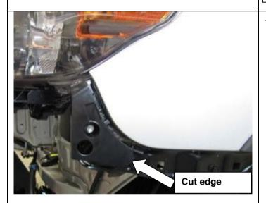
28. Once cut, replace forward section only of clip to vehicle as shown
